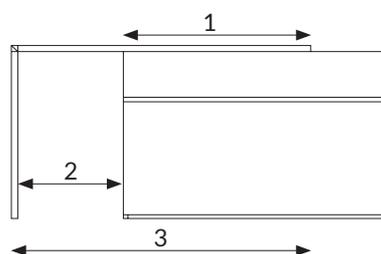
1. The part of the add-on top based on the counter must be at least 600 mm long.
